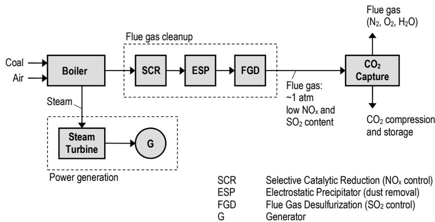
Fig. 2 – Coal-fired power plant with post-combustion CO<sub>2</sub> capture.
