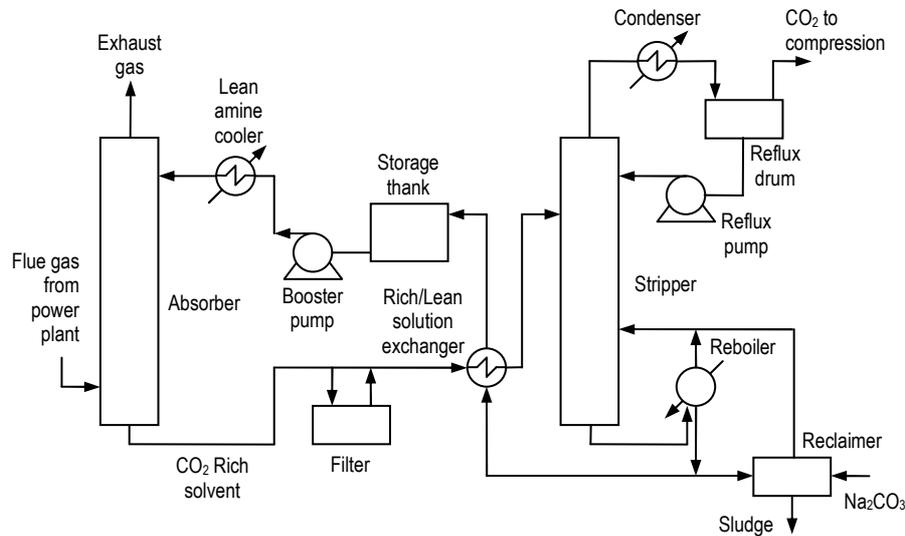
Fig. 3 – Process flow diagram of an amine-based system.
